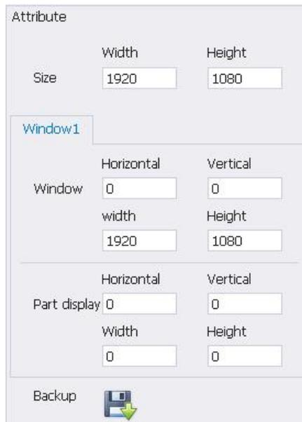
The property parameters include screen point settings, window size and position settings, local display size and position settings, and a backup button for system data backup.
