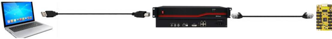
③ Use only the receiving card: The computer and the receiving card are connected via a network cable.
