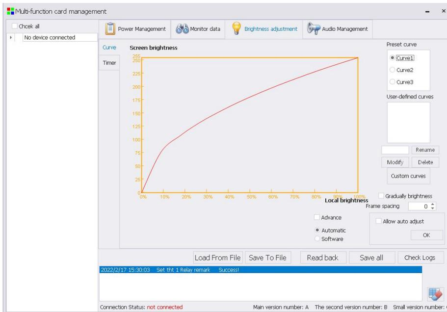
Through the external light sensor device, the curve can be set in the brightness adjustment interface (horizontal coordinate is the brightness of the large screen, the vertical coordinate is the ambient brightness), and the brightness of the large screen can be adjusted according to the ambient brightness detected by the light probe.
