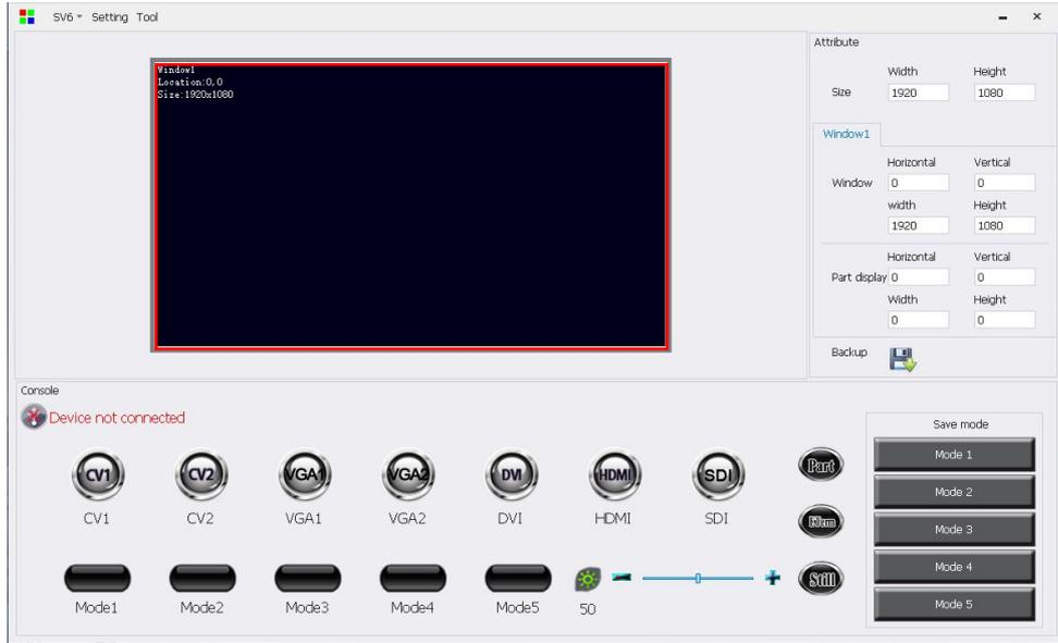
The simulation operation area can display the screen window number, screen position, and screen size information, and supports dragging and dropping the screen within the range of screen points.
