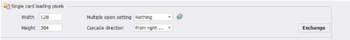
The single card load information section contains the single card load information of the receiving card, and the load information, multi-open mode, module cascade direction, and data group exchange of the receiving card can be adjusted through this part.
