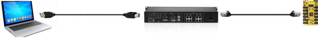
② Use the sending device and the receiving card: The serial port connection between the sending device and the computer, and the sending device and the receiving card are connected through the network cable.
